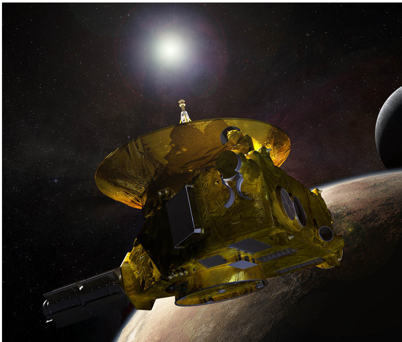
Figure 1.14: Artist's rendition of New Horizons approaching Pluto. New Horizons is a spacecraft originally designed to conduct the first flybys of Pluto and a Kuiper Belt object. It is currently conducting its second extended mission from its location in the outer Solar System at 58 au. (Image: Johns Hopkins APL.)
