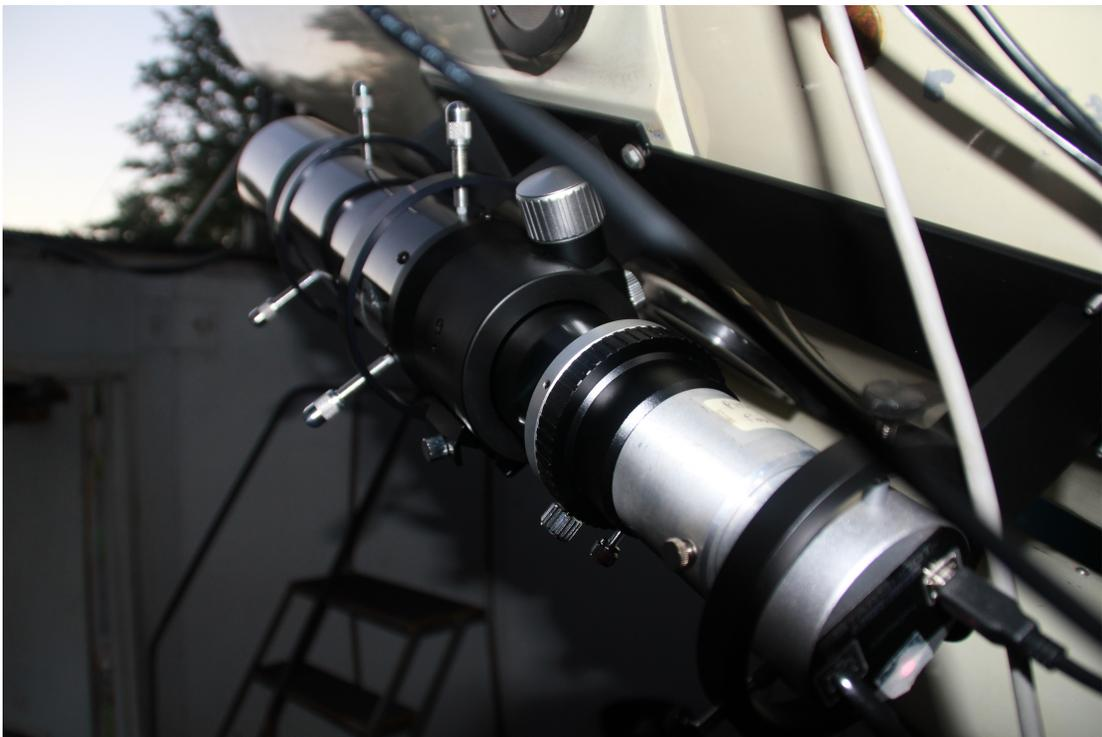
**Figure 3.1:** The final setup of the autoguider.
