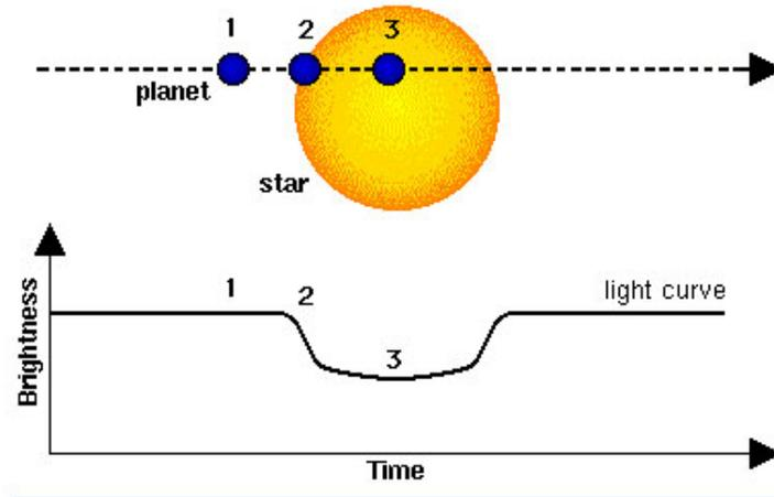
**Figure 1.1:** A schematic of an exoplanet transit (CNES, 2010).
