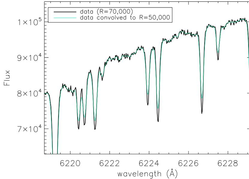
**Figure 4.6:** An example of how the convolution affected the data. As expected, adjusting the resolution of the data down to a common level caused the absorption line depths to be a bit shallower. Since precise line depth measurements is paramount for our analysis, this was an important step to get right!
