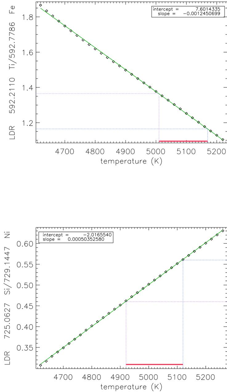
**Figure 6.1:** These are the monotonic plots from Figure 4.12 with the temperature range (pink) corresponding to the ratios (with the exception of one outlying point) from Figure 5.3. The temperature ranges indicated by the two ratios do not exactly match, as we would hope, but they do overlap, which is encouraging for our future analyses.
