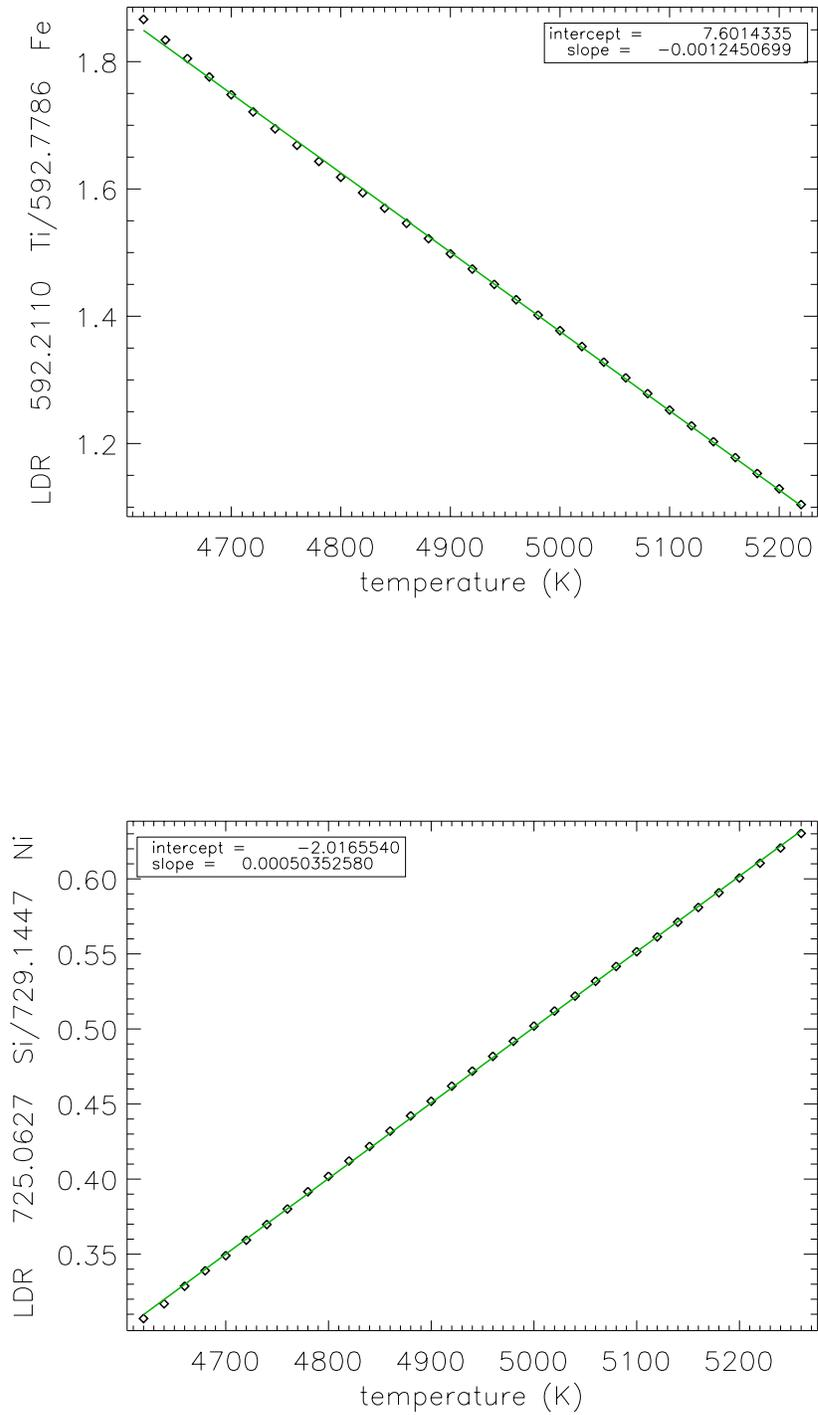
**Figure 4.12:** The temperature sensitivity of two LDRs.
