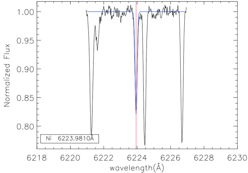
**Figure 4.2:** An example of continuum normalization. Our line depth measurements were made using the normalized spectra.
